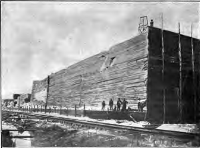
FIG. 67. — A solid block of Louisiana sulphur. Molten sulphur is pumped from wells into immense wooden bins, where it solidifies. It is then broken by blasting and loaded on freight cars for shipment.
